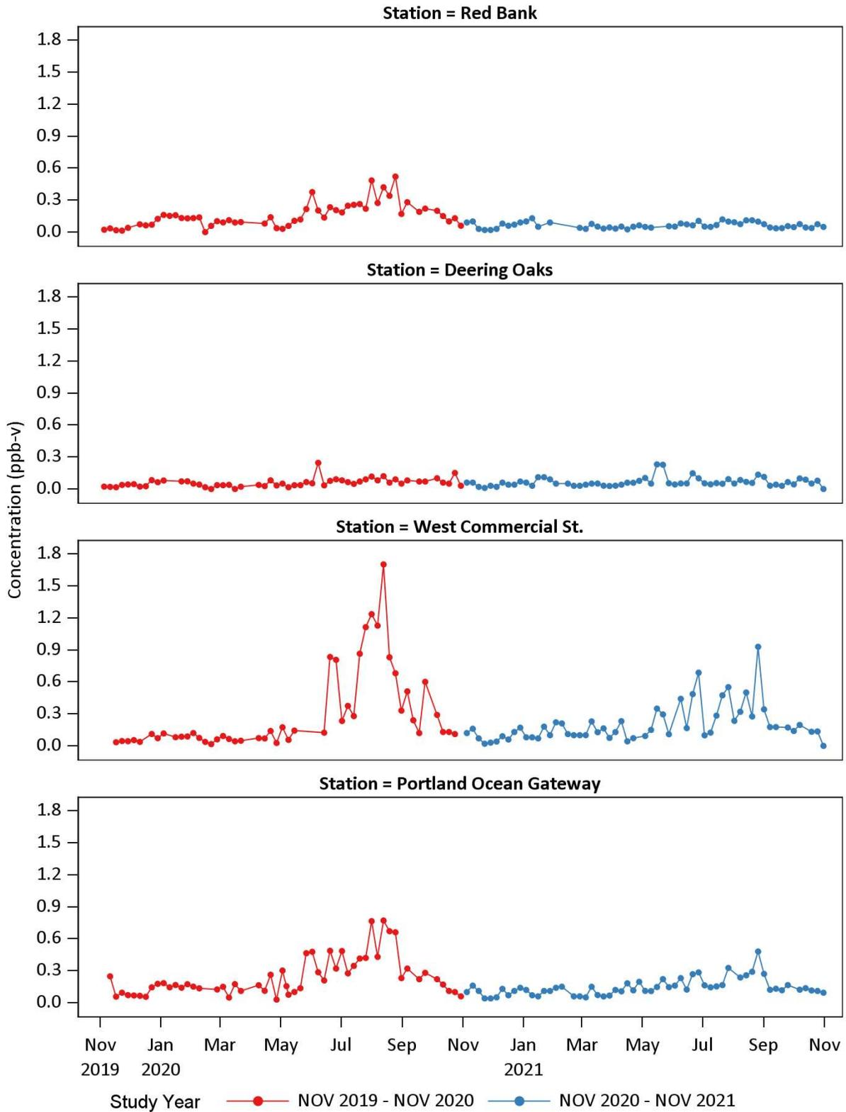
Figure 9 shows the individual 24-hour sample results in the first (red) and second (blue) full year of monitoring for naphthalene for each of the original 8 stations. 24-hour air samples are collected every 6 days. Sampling data obtained from Maine DEP. Central Receiving taken offline March 17, 2021; Mechanic Street (not included) brought online March 23, 2021.
