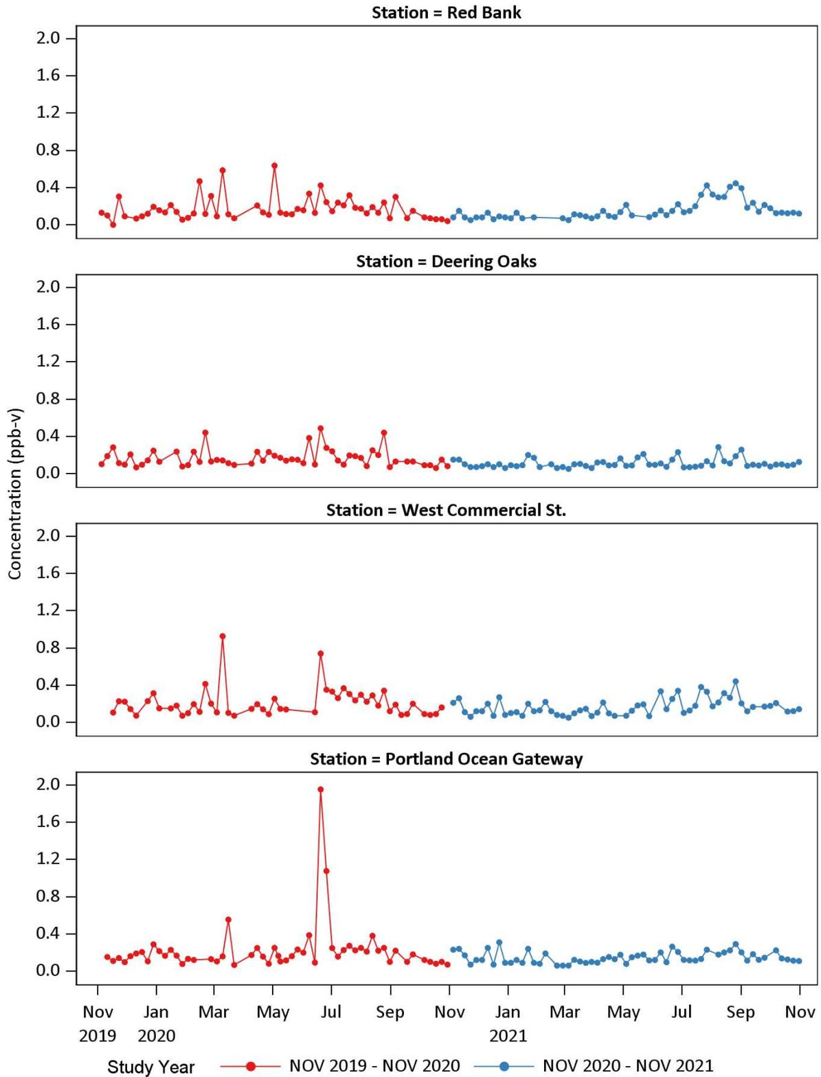
Figure 7 shows the individual 24-hour sample results in the first (red) and second (blue) full year of monitoring for acrolein for each of the original 8 stations. 24-hour air samples are collected every 6 days. Sampling data obtained from Maine DEP. Central Receiving taken offline March 17, 2021; Mechanic Street (not included) brought online March 23, 2021.
