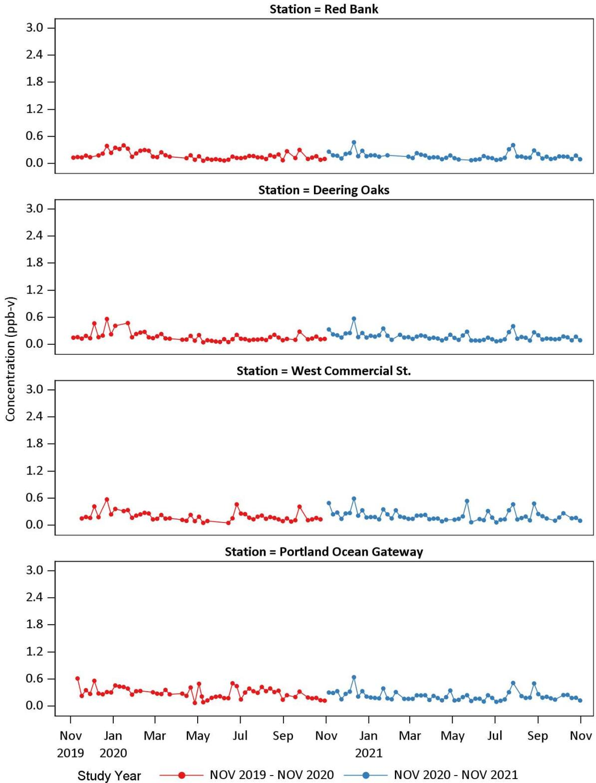
Figure 8 shows the individual 24-hour sample results in the first (red) and second (blue) full year of monitoring for benzene for each of the original 8 stations. 24-hour air samples are collected every 6 days. Sampling data obtained from Maine DEP. Central Receiving taken offline March 17, 2021; Mechanic Street (not included) brought online March 23, 2021.
